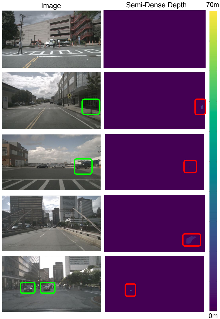
Figure E. Failure modes for our RadarNet model (best viewed in color at 4x). The figure shows (L-R) the camera image, and the quasi-dense depth (output of the RadarNet). The range of depth is between 0-70m (as shown in the colorbar on the right). We mark the errors with red boxes and the corresponding objects in the image with green boxes.
