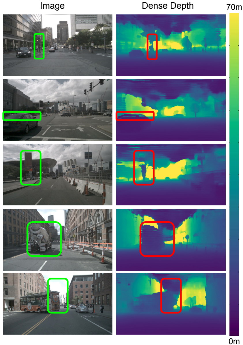
Figure F. Failure modes for FusionNet model (best viewed in color at 4x). The figure shows (L-R) the camera image, and the predicted dense depth (output of the FusionNet). The range of depth is between 0-70m (as shown in the colorbar on the right). We mark the errors with red boxes.
