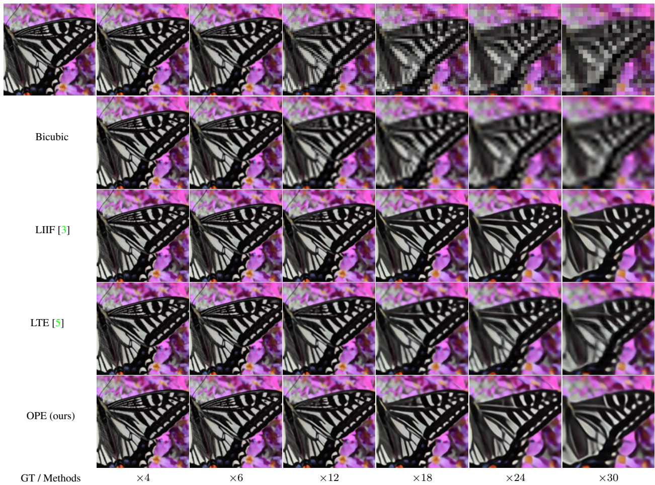
Figure 3. Qualitative comparison with SOTA methods for arbitrary-scale SR. On div2k 0882.png. 1-st row: ground truth, input images with different scale factor (larger scale factor to lower resolution).
