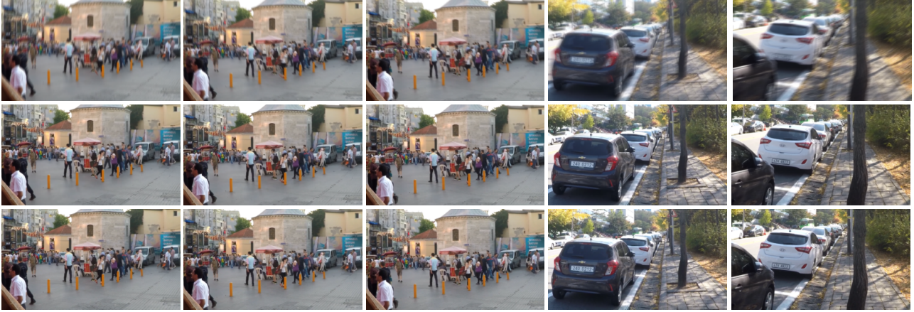
Figure 13. Additional event-based single image deblurring results of our REFID on the test set of GoPro. From top to bottom: blurry image, result of REFID, ground truth.
