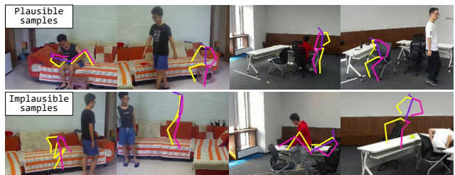
Figure 1. Samples used to develop the semantic score classifier. Plausible ones are samples in the dataset, while implausible ones are derived by random pose replacement, shift, and perturbation.
