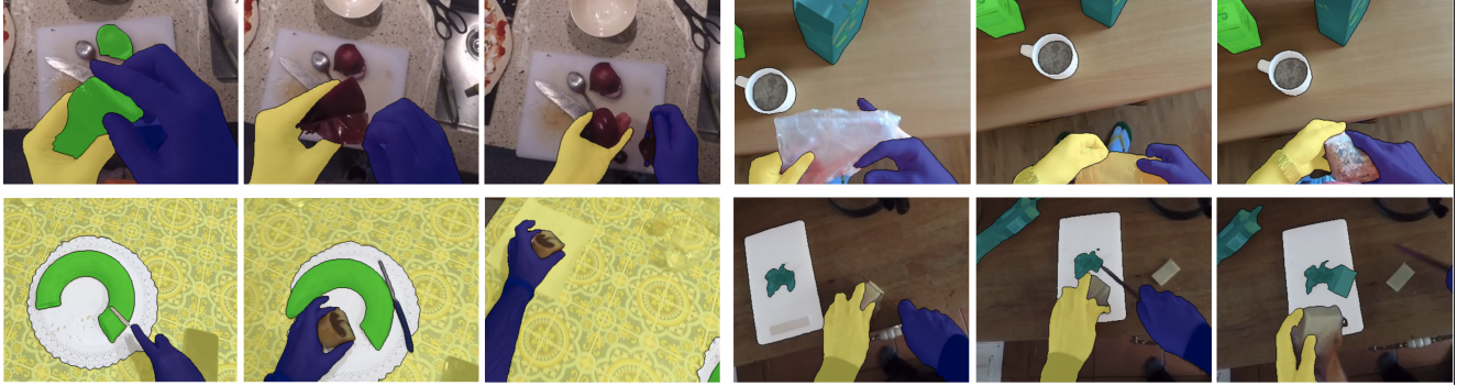
Figure 5. Visualization of automatically interpolated and filtered VISOR labels [5]. Colours indicate instance ids. We can see that automatic interpolation fails during transformations, such as peeling of the onion or folding of the cereal bag in the top row, whereas the objects with stable appearance, such as hands or boxes on the table are perfectly segmented. In VOST we are focusing precisely on the scenarios that automatic interpolation cannot handle, justifying our decision to densely label videos at 5 fps.
