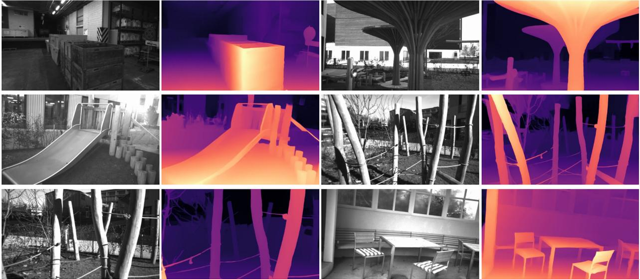
Figure 14. **Qualitative results on ETH3D.** We show reference images and disparity maps predicted by our NS-RAFT-Stereo.
