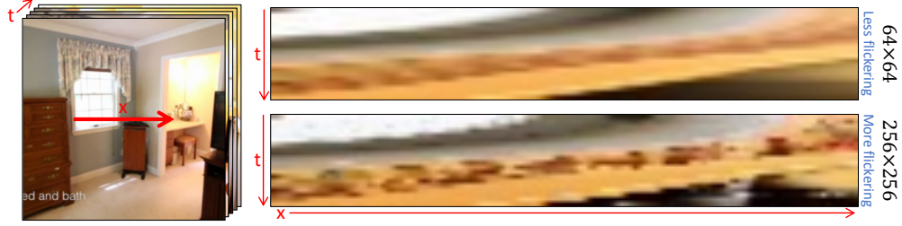
Figure 2. X-T slice visualization. We visualize the x-t slice of the low-resolution ( top ) and high-resolution ( bottom ) videos. The flickering mainly comes from the super-resolution stage.
