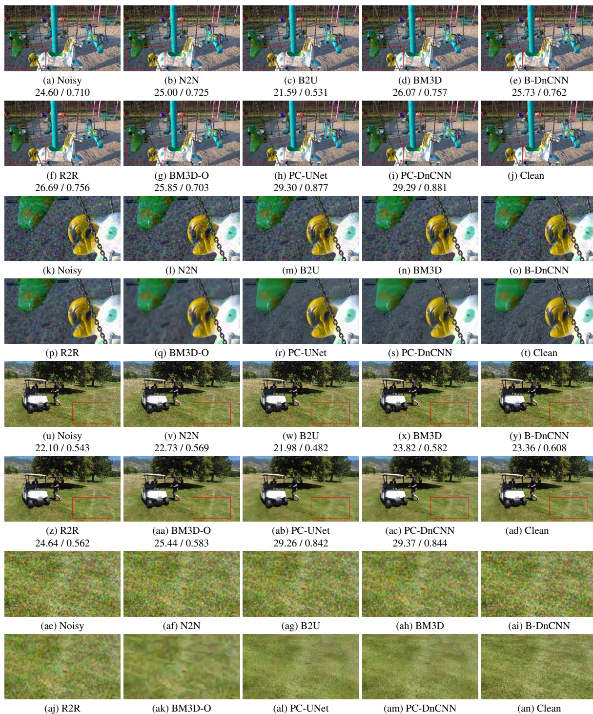
Figure 3. Denoising examples with correlated Gaussian noise. The first four rows show frame 5 of the sequence carousel with \sigma = 15 and k = 4 . The last four rows present frame 13 of the sequence golf with \sigma = 20 and k = 4 . As can be seen, oracle BM3D produces blurred images while leaving a substantial amount of low-frequency noise unfiltered. Other algorithms, except ours (PC-UNet and PC-DnCNN), do not succeed in removing the noise.
