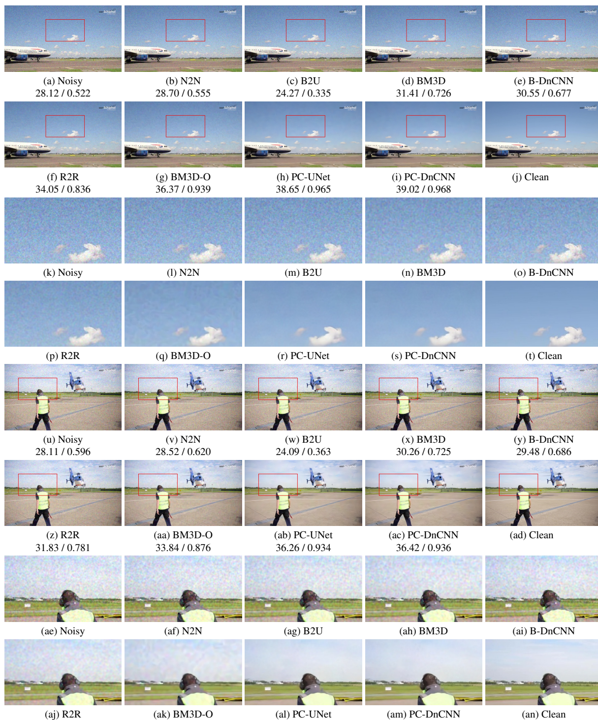
Figure 2. Denoising examples with correlated Gaussian noise. The first four rows show frame 13 of the sequence planes-crossing with \sigma = 10 and k = 3 . The last four rows present frame 5 of the sequence helicopter with \sigma = 10 and k = 4 . As can be seen, oracle BM3D leaves a substantial amount of low-frequency noise unfiltered, while other algorithms, except ours (PC-UNet and PC-DnCNN), do not succeed in removing the noise.
