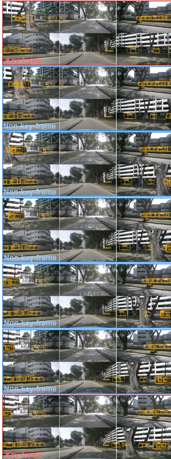
Figure 2. Visualization of the surround-view annotation in nuScenes-H, where the key-frames are the 2Hz images in the original nuScenes dataset [1], and the intermediate non-key-frames are the annotated 12Hz images.
