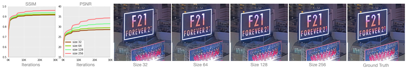
Figure D. The ablation study results for the MLP size. As the MLP size increases, the network becomes better at composing signals from various levels, thus various frequencies, leading to a better final outcome.
