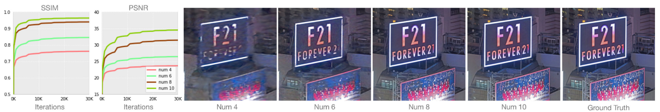
Figure E. The ablation study for the number of levels for the Fourier grid feature. More levels lead to a drastic increase in the quality of fine details.
