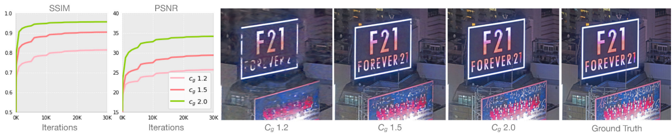
Figure C. The ablation study for the scaling coefficient c_g . With larger c_g , reconstruction quality improves, with more fine details being preserved and with higher spatial resolution.
