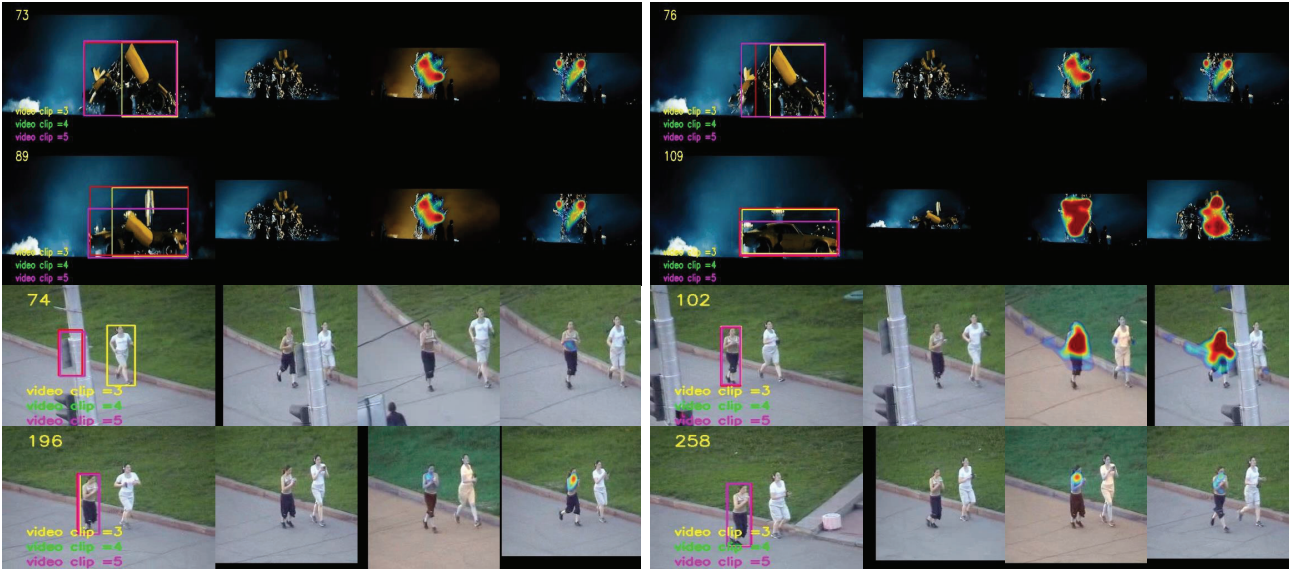
Figure 2. Visualization results of the three VideoTrack settings: the lengths of input sequence are set to 3, 4 and 5, respectively. The frame in second column is the nearest intermediate template t_T whose the center point performs as the query for the cross attention. The third and fourth row are another two intermediate templates t_{T-1} and t_1 , respectively.
