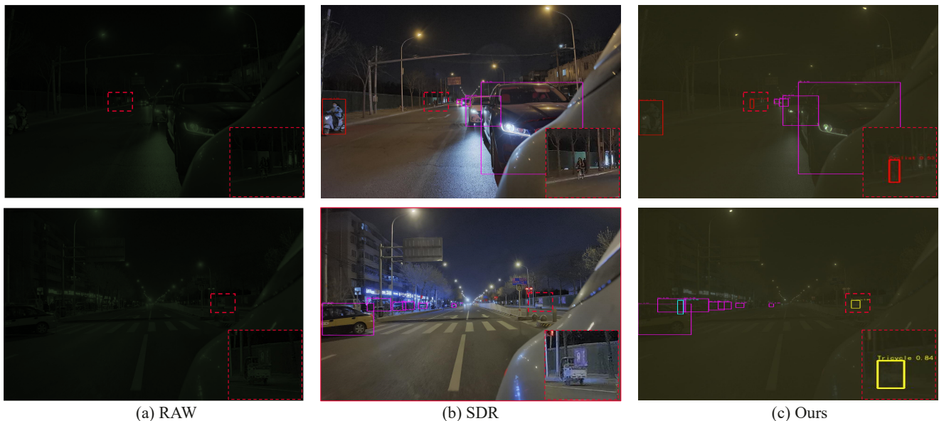
Figure 2. Visual examples of object detection on the night scene of the ROD dataset. (a), (b) and (c) are results of RAW data, SDR data and our method, respectively. Our method significantly outperforms the SDR data. Please zoom in for confidence scores and class predictions.
