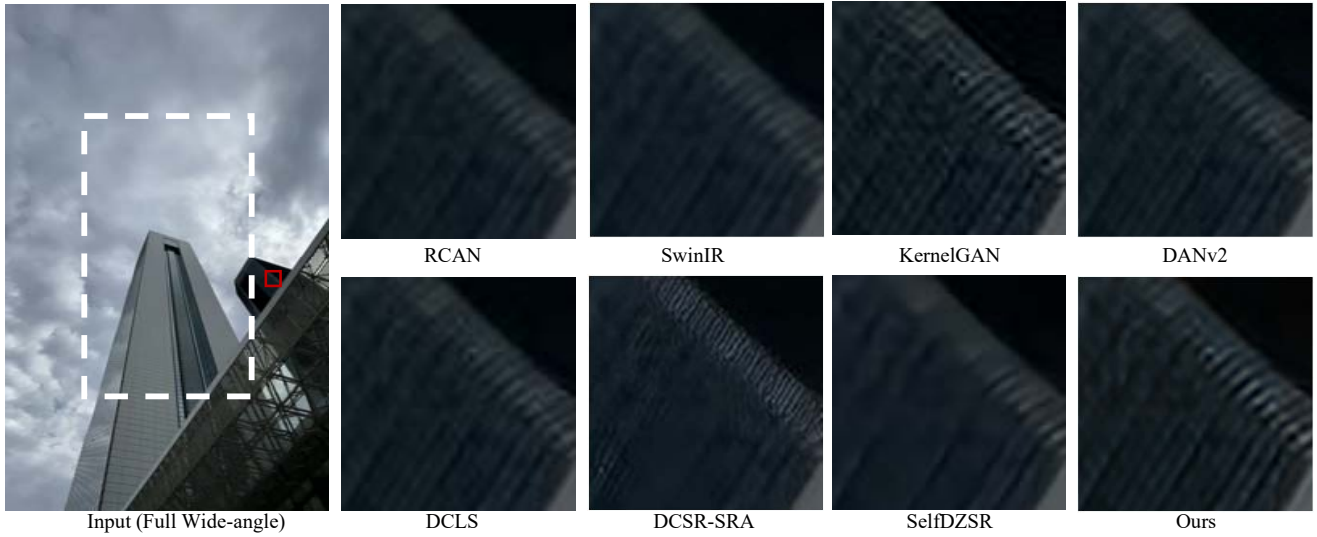
Figure 7. Visual comparisons for 2\times SR on real-world data captured by iPhone12. The white dotted box indicates the overlapped FoV.
