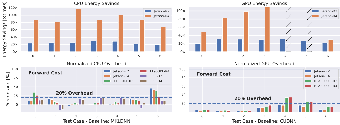
Figure 11. Energy savings and overhead results on multiple CPUs and GPUs under different test cases ( i.e. , different input sizes, number of channels, etc.). For test case 4 and 5 with patch size 4 \times 4 (Jetson-R4) on GPU, the latency of our method is too small to be captured by the power meter with a 20 ms sample rate so the energy savings data is not available. For most test cases with patch size 4 \times 4 , our method achieves over 80\times energy savings with less than 20% overhead.
