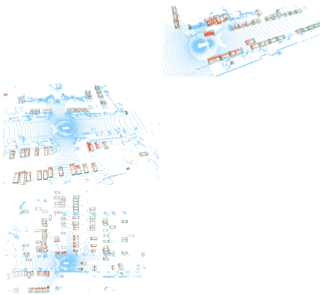
Figure 2. Visualization of detection results on the Waymo validation set. We show the raw point cloud in blue, ground truth in green bounding boxes, our detected objects in gray bounding boxes, and points inside our detected boxes in orange.
