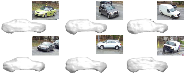
Figure 1. Vehicle Category Reconstruction. Our method is able to fuse videos of 365 vehicles with different appearance and shape into a category model. From left to right, we show reconstruction of sedans, SUVs, and vans.
