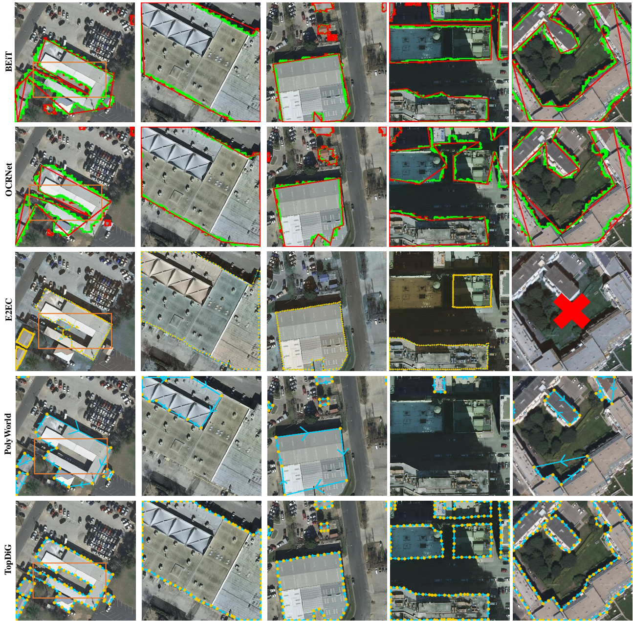
Figure 2. Visual comparisons on the polygon-shape targets. These images come from the Inria dataset. Top - bottom: BEiT, OCRNet, E2EC, PolyWorld and TopDiG. Green line: segmentation contours of buildings; Red line: simplified polygons using the DouglasPeucker algorithm; Yellow dots: detected/sampled nodes; Cyan arrow lines: directional connections between node pairs; Red cross: no predicted building; Orange rectangles: concave building outlines.
