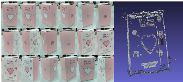
Figure 6. Object reconstructed by VisualSFM and PMVS2. Selected multi-view image inputs are shown on the left and reconstructed dense point clouds are on the right.
