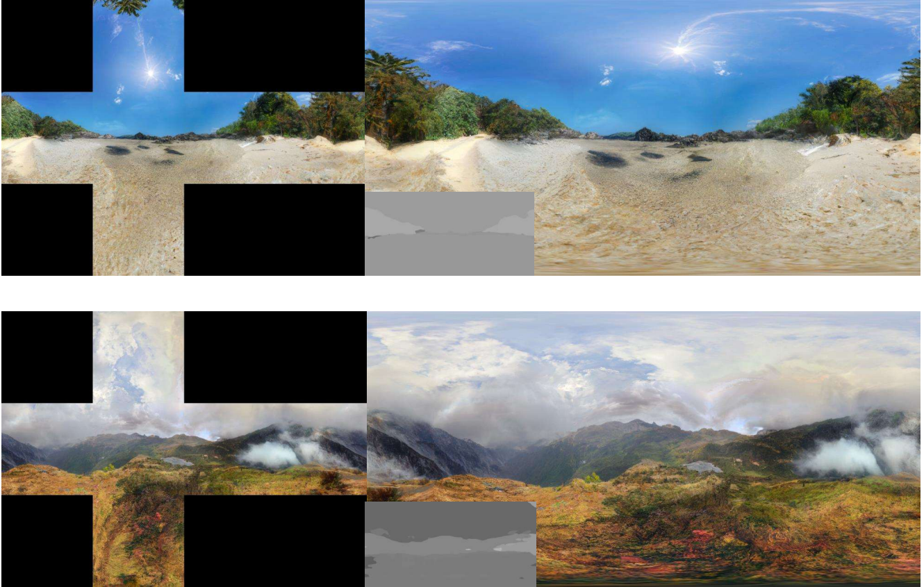
Figure 16. DiffCollage on 360 cubemap image. (Left) Cubemap representation; (Right) Equirectangular representation; (Lower middle) Semantic segmentation map used to condition the model.
