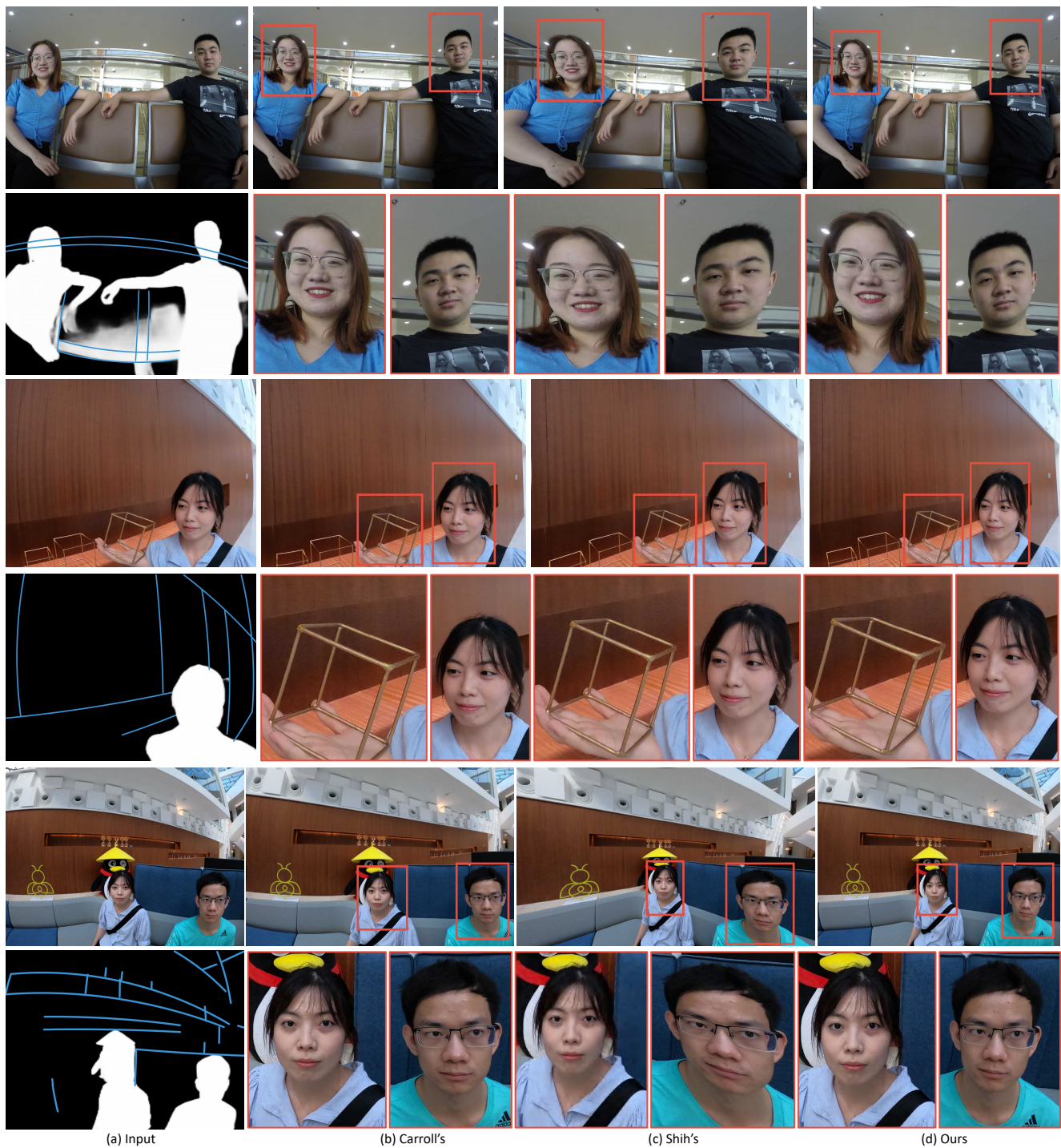
Figure S9. Comparison in detail. (a) shows the input of the proposed method, including the wide-angle image and visual features of image content analysis. (b-d) show the rectification results of Carroll's, Shih's and our methods. Compared with state-of-the-art methods, our method has effectively removed the wide-angle distortions while at the same time maintaining an ultra-wide field of view, without sacrificing salient image contents.
