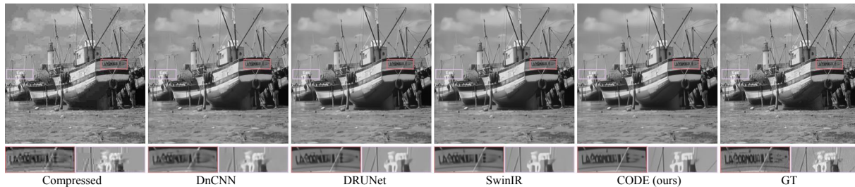
Figure 16. Qualitative comparisons of JPEG compression artifact reduction (compression level q = 10 ) on the Classic5 dataset.
