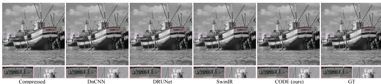
Figure 19. Qualitative comparisons of JPEG compression artifact reduction (compression level q = 40 ) on the Classic5 dataset.
