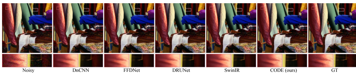
Figure 11. Qualitative comparisons of color image denoising (noise level 15) on the McMaster dataset.
