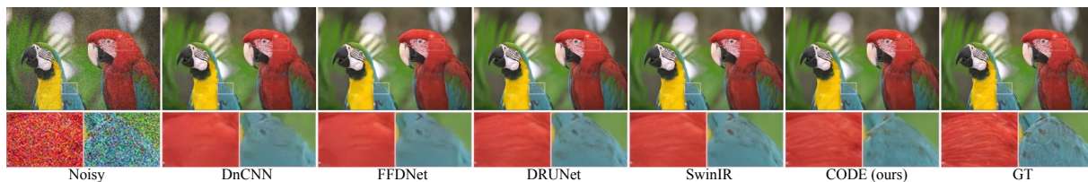
Figure 10. Qualitative comparisons of color image denoising (noise level 50) on the Kodak24 dataset.
