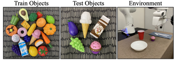
Figure 8. Objects used for the real-world object generalization experiment. Given a training set of grasping demonstrations with 20 objects (left), we evaluate policies against 5 held-out test objects (middle). All demonstrations and evaluations are completed on a tabletop with randomly positioned distractor objects (right).
