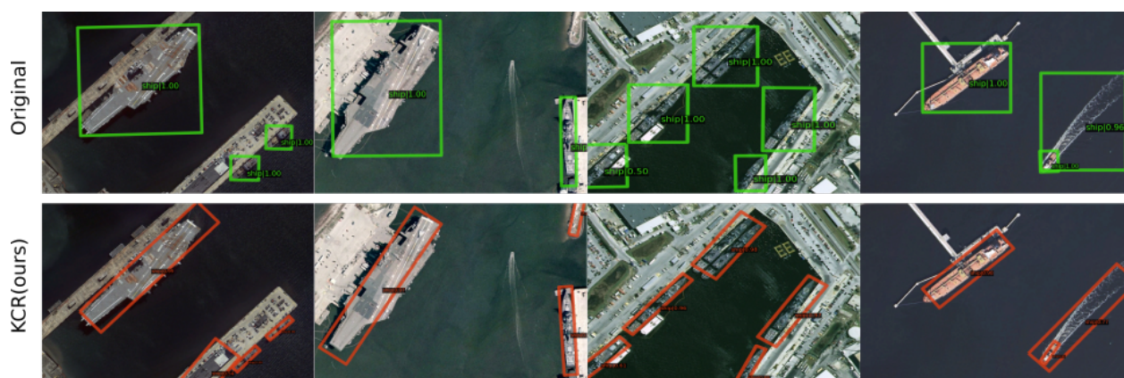
Figure E4. Failure cases of KCR. For the first two cases, some KCR rotated boxes are not tight. But they are still much tighter than axis-aligned boxes. For last two cases, KCR either detects two ships as one or detects the ship trace. Original detector also fails in those two cases.
