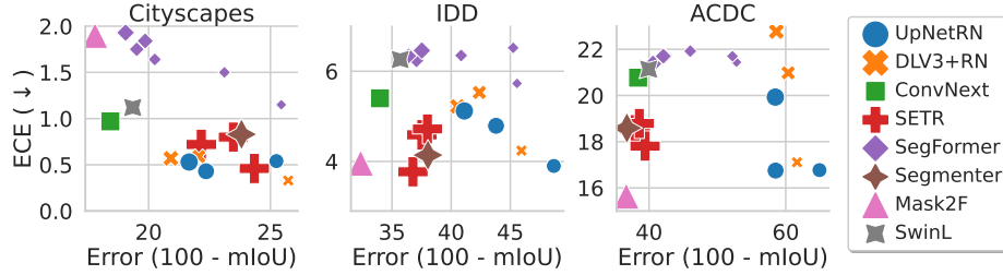
Figure 18. mIoU error (↓) vs. Expected calibration error (↓) . All models were trained on CS. Markersize proportional to number of parameters. Interestingly, we observe that Mask2Former seems to be the best-performing model in terms of mIoU in all datasets. In terms of calibration error Mask2Former is poorly calibrated in distribution (CS) but has a milder increase in ECE as the distribution shift becomes stronger.
