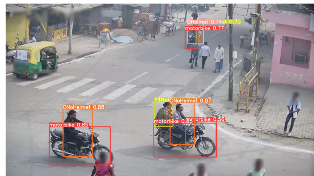
Figure 1. Illustration of predictions of motorists, passengers, and motorcycles in real-time. We present a method that is able to predict helmet rule violation in real-time. The different bounding box colors represent different predictive class.
