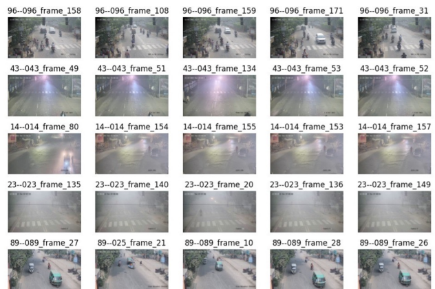
Figure 6. Clustering of frames with high similarity. Each row represent frames of high similarity.
