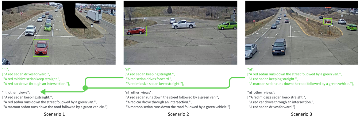
Figure 2. The different video frames and NL descriptions of the same vehicle in the CityFlow-NL train dataset. In the NL descriptions, tracked-vehicle color, type, motion, and other surrounding vehicle information are provided. Some NL annotations from other camera views are arranged in the NL other views.
