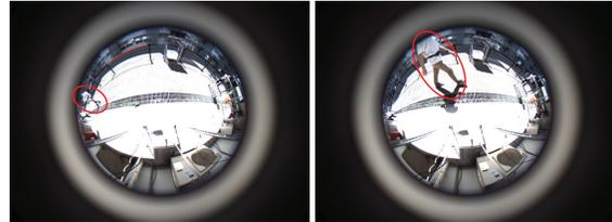
Figure 1. Gait image examples captured by a fisheye camera. The person circled in red is the walking subject. Because the camera height is set relatively lower, the occlusion increases as he approaches the camera. In addition, there are severe distortions in the fisheye images.
