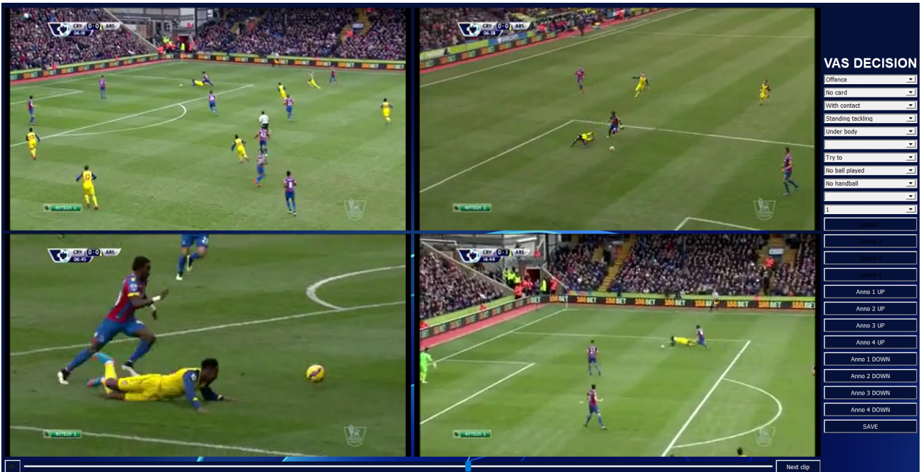
(a) VARS annotator. The annotator may browse simultaneously the synchronised videos either at regular speed or frame by frame. He can annotate all 10 properties and adjust the annotated point of contact for each clip separately and temporal align the different clips by modifying the speed and offset of the clips.
