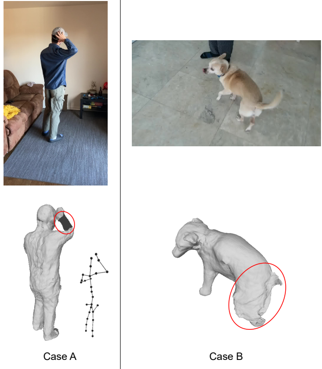
Figure 4. Failure case examples. In Case A, the mesh of the person’s right arm collapses despite the kinematic chain being able to represent the correct pose. In Case B, the dog’s tail and back legs are missing due to bad reconstruction.
