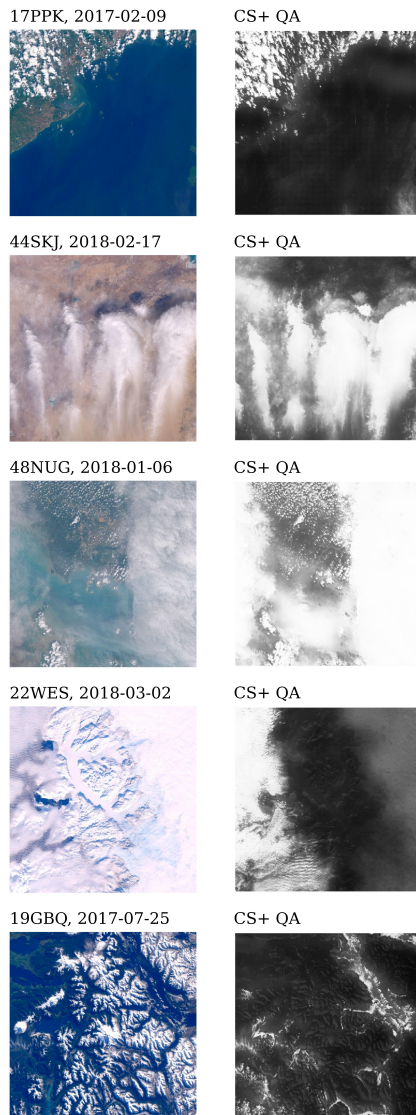
Figure 5. Sentinel-2 L1C images and corresponding Cloud Score+ QA results for six images from the CMIX-I PixBox dataset.
