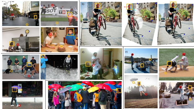
Figure 2. Visualisation of different failure cases , including human bias (a), ground truth annotation ambiguity (b), occlusion of the subject (c) and the gaze target (d), and physically impossible estimates (e). The observed subject’s head bounding box is highlighted in yellow, the ground truth annotation is marked as a yellow circle or blue dot, and the estimated gaze target estimate is shown as a red circle.
