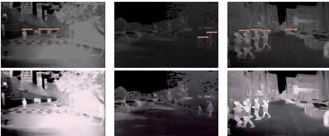
Figure 9. Examples of pedestrian detection using YOLOv7 on KAIST dataset with and without TE-VGAN.
