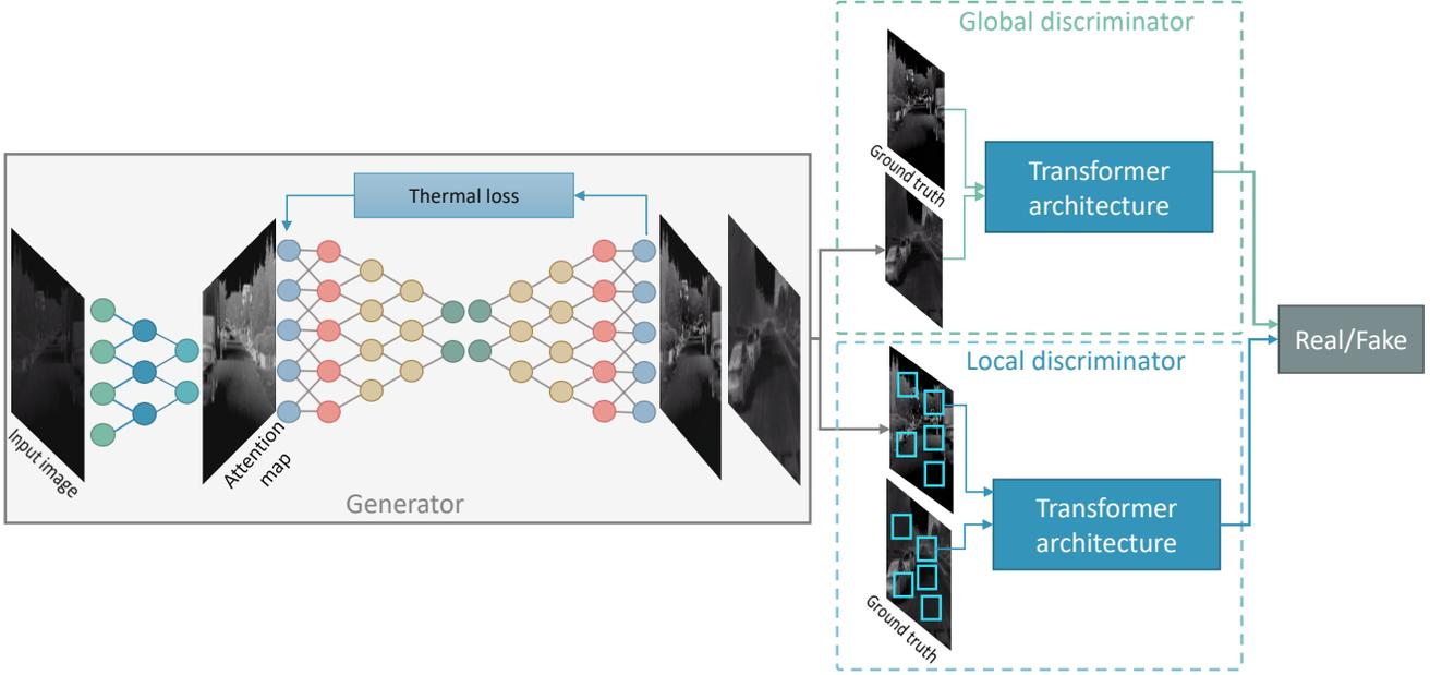
Figure 3. The proposed TE-VGAN architecture composed of generator and two ViT discriminators.
