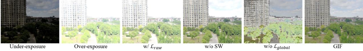
Figure 7. Visualization of the ablation results over the core components within the GIF. Three groups of control experiments are carried out: 1)  $w/ \mathcal{L}_{raw}$ : utilize the unprocessed raw gradient map as  $\{w_i\}_{i=0}^1$ ; 2)  $w/o$  SW: substitute the saturation-based weighting (SW) in  $\mathcal{L}_{smooth}$  with a simple weighted average operation; and 3)  $w/o \mathcal{L}_{global}$ : without the devised artifacts removal-oriented global constraint.
