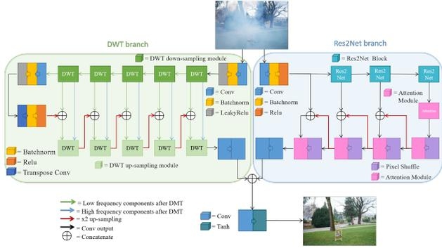
Figure 6. The network architecture of the solution proposed by team NTU607-dehaze.
