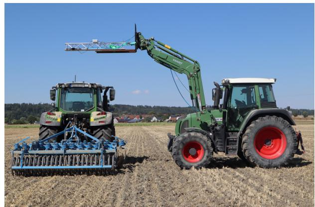
Figure 2. Dust measurement setup with a boom attached to a front loader, and a second tractor with a disc harrow.
