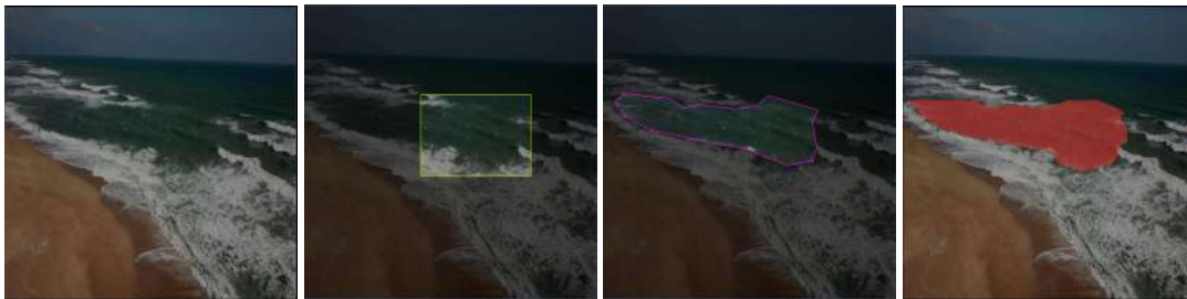
Figure 1. An illustration of a visible rip current and its detection task, displayed from left to right: 1. The original photo, 2. The bounding box annotation from the YOLO-Rip dataset, 3. Our ground-truth annotation for instance segmentation, 4. Prediction using YOLOv8. This example highlights how bounding boxes may exclude relevant parts of the rip currents while also incorporating surrounding noise.
