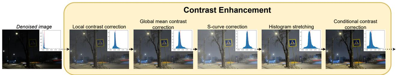
Figure 5. Analysis of the results obtained after each operation within the contrast enhancement step of our pipeline. Image histograms show how global contrast changes after each step.
