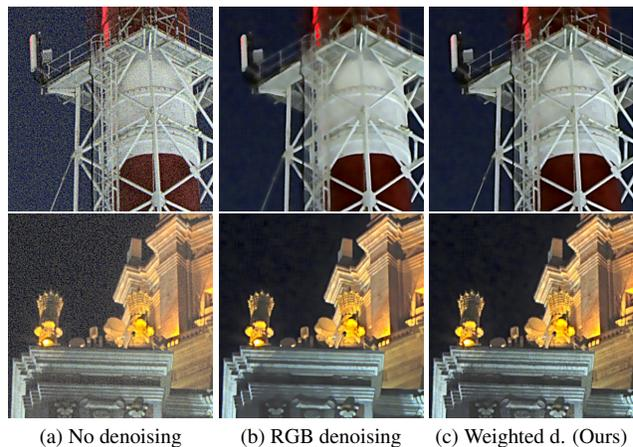
Figure 4. Analysis of the denoising operation. Applying denoising to RGB channels leads to a heavier loss of details (Figure 4b). The adopted solution applies stronger denoising to chroma channels than to the luminance channel (Figure 4c).
