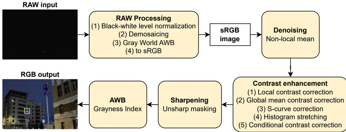
Figure 2. Overview of the proposed ISP pipeline for night photography rendering.
