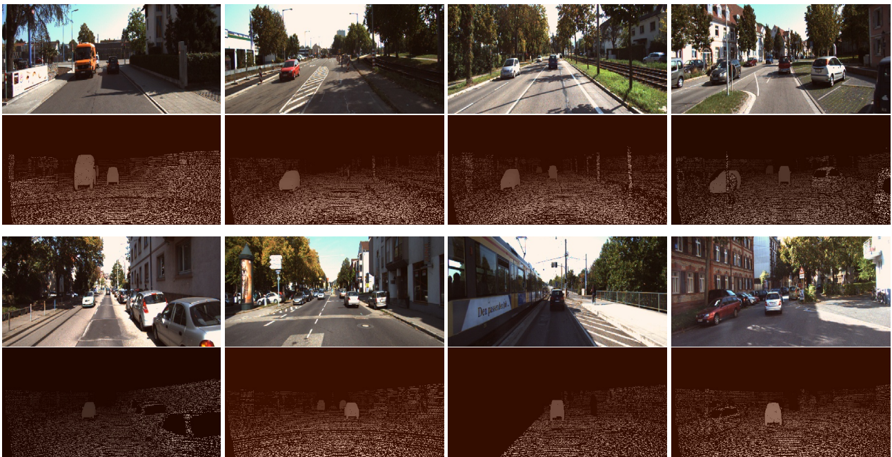
Figure 3. Disparities of example videos from KITTI stereo 2015 [5] (rows #1 and #2) and 2012 [3] (rows #3 and #4) datasets. The salient object (cars) are apparent in the disparity maps, but they could not be used as the saliency detection method because of the high disparity values of near objects.
