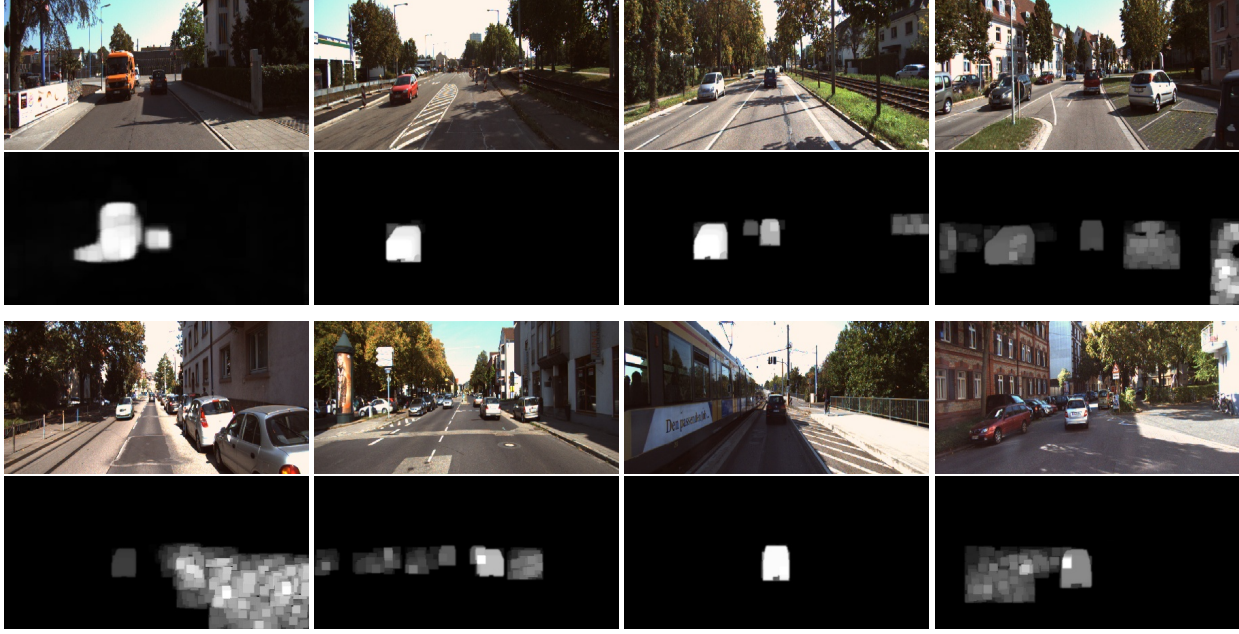
Figure 4. Saliency objects detected using the combination of CoSD, Yolov5, and disparity.
