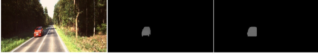
Figure 11. Dilation of the salient region. It helps to enlarge the object to warp without changing its shape.
