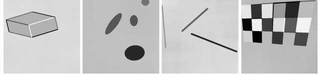
Figure 2. Synthetic images with geometric primitives. Image samples of size 320 \times 320 created at runtime to pre-train the interest point detector pipeline.
