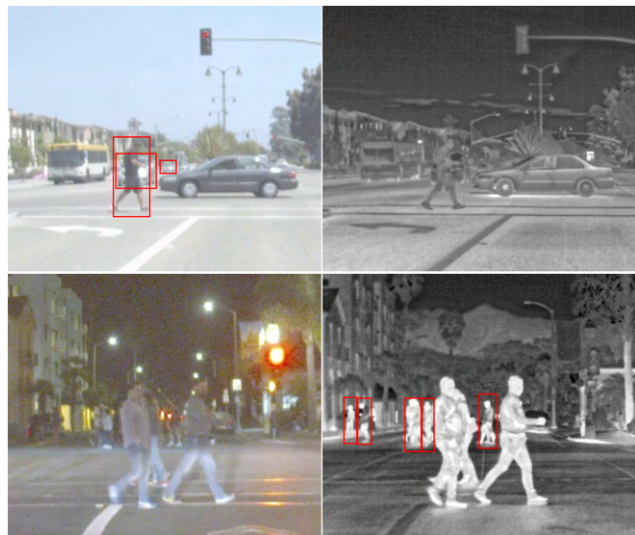
Figure 1. Daytime (top row) and nighttime (bottom row) samples from the FLIR dataset [30]. Objects in the bounding box indicate that the current modality can obtain more details and can be used as a complement to another modality.
