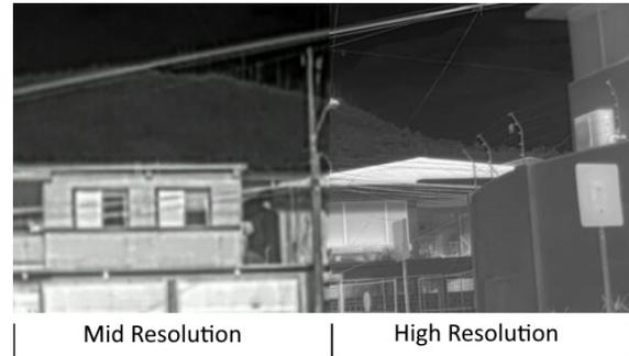
Figure 1. A montage of two thermal images captured from the same point of view but with different cameras at different resolutions. The (left) image is a crop from the MR image, while the (right) image is a crop from the HR image [11].
