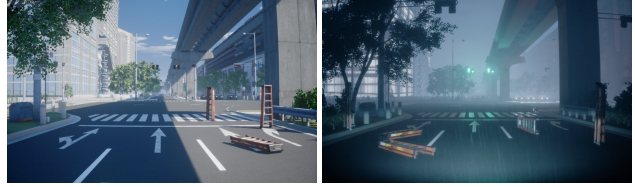
Figure 4. Examples of spawned ladder models using domain randomization with different times of day and weather conditions.
