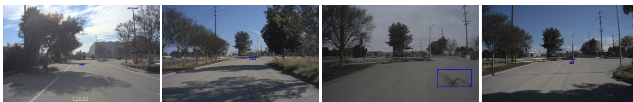
Figure 10. Detections of unseen road debris using HazardNet. Ground truth labels are drawn in blue, and HazardNet detections are drawn in red. The network is able to detect debris missed by human annotators (row 3, columns 3 and 4).
