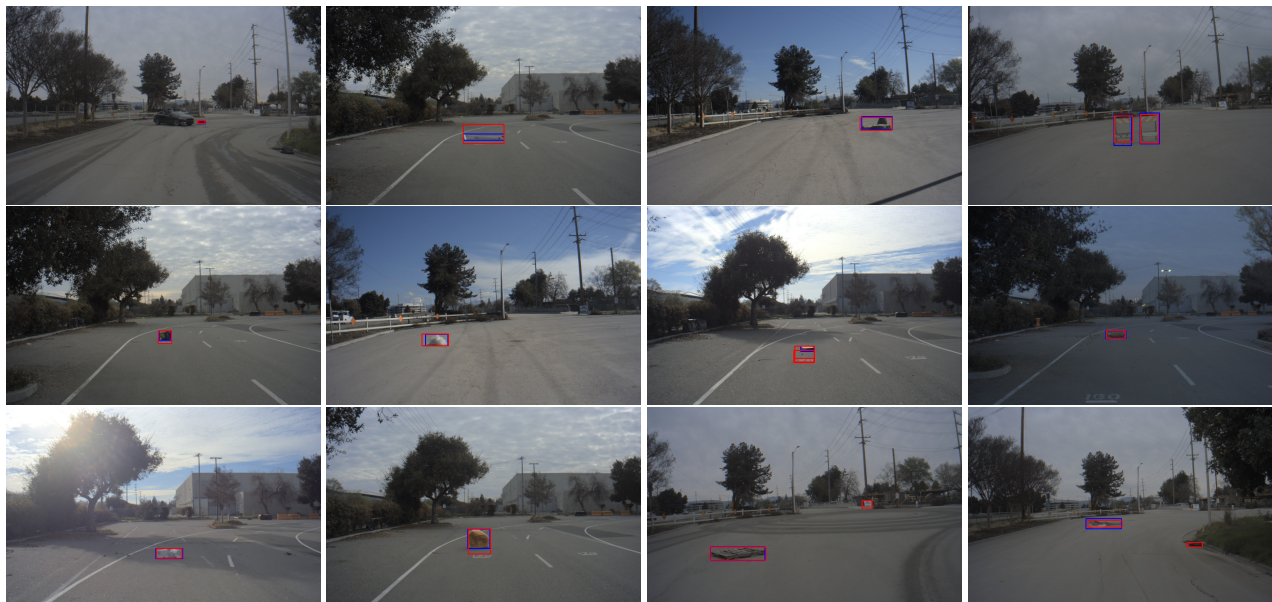
Figure 10. Detections of unseen road debris using HazardNet. Ground truth labels are drawn in blue, and HazardNet detections are drawn in red. The network is able to detect debris missed by human annotators (row 3, columns 3 and 4).
