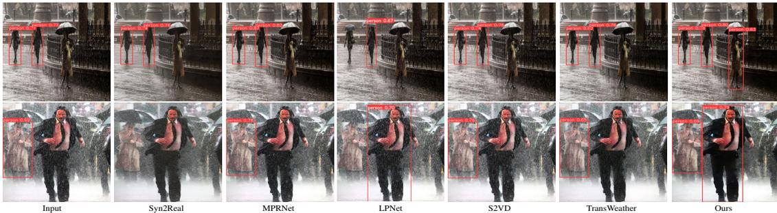
Figure 6. Sample results of object detection using YOLOv5 model after deraining using various algorithms. We show that even in the case of partial deraining during heavy rainfall (bottom row), the detection confidence increases.
