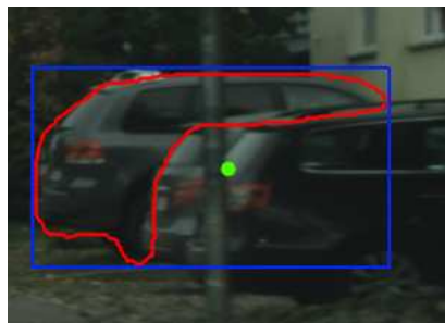
Figure 9. Example of polygon polar origin finding. If the vehicle object is partially occluded, the bounding box center (green) is outside of the polygon shape boundary (red).
