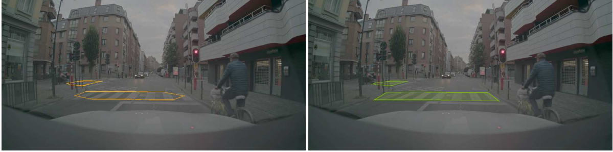
Figure 7. Two examples to visualize 64-vertex PolarMask (left) and 36-vertex DPPD (right) results on crosswalks. DPPD expenses less vertices but achieves tighter alignment with the groundtruth.
