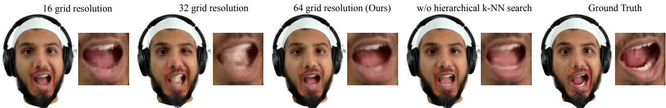
Figure 6. Qualitative results of using different 3D grid resolutions during hierarchical k -NN search and without hierarchical k -NN search for ablation studies. “ 16 grid resolution ” results in blocky artifacts around mouth and nose. “ 32 grid resolution ” removes blocky artifacts, but produces floaters inside mouth. “ 64 grid resolution ” produces a similar level of visual quality as “ w/o hierarchical k-NN search ”.
