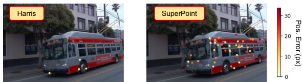
Figure 9. Existing keypoint selectors either offer a sparse set of options (Harris) or fail to avoid regions with visual imperfections (SuperPoint).
