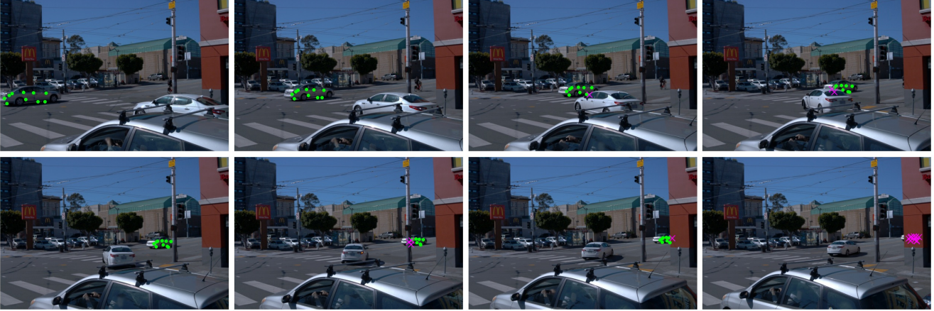
Figure 5. Visible point correspondences (●) and occlusions (×) computed by DriveTrack over eight samples from a 30-frame sequence.
