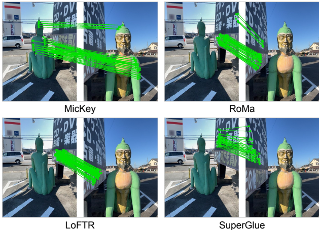
Figure 5. MicKey establishes keypoint correspondences even though images share very little visual overlap. Contrary to other matchers, MicKey does not focus on the textured wall, but instead reasons about the shape of the object in the foreground.
