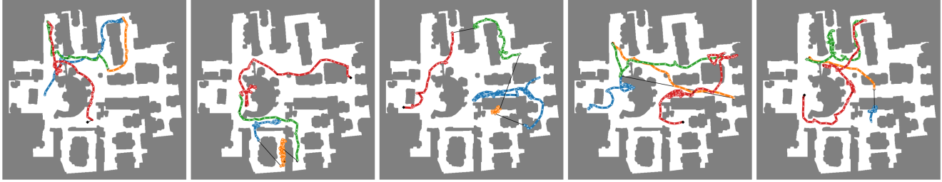
Figure 7. The 20 trajectories of \overline{\text{Office/20}} are distributed over 5 plots and superimposed on the map, color coded. If an episode fails, the remaining distance is shown as a straight black line from the last position to the goal. The agent is variant \beta of Table 4.
