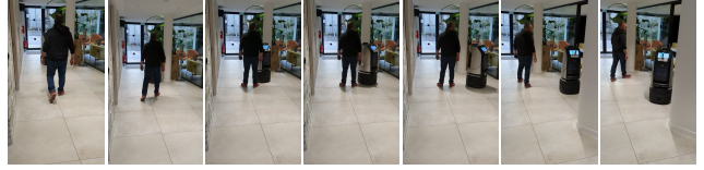
Figure 6. Dynamic obstacles: our agent stops and circumvents people, achieved through a highly negative collision reward term.
