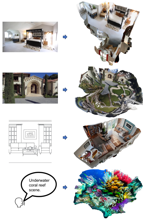
Figure 8. 3D point cloud generation. Performing depth estimation on the generated panorama further enables the creation of 3D point clouds from diverse inputs. We can generate point clouds for both indoor and outdoor scenes, even the underwater scene with clear geometry of the fishes and coral reefs.
