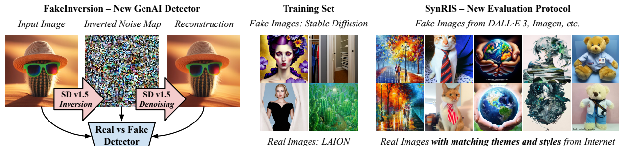
Figure 1. (left) We propose a new synthetic image detector that uses two additional input signals derived from a fixed pre-trained Stable Diffusion [45]: an inverted latent noise map and the reconstructed input image. (middle) Our detector is trained using fake images generated using Stable Diffusion and real LAION images. It achieves state-of-the-art generalization performance in detecting unseen text-to-image generators. (right) To ensure that the performance evaluation does not favor detectors that are biased towards particular themes or styles, we introduce a new thematically and stylistically aligned evaluation benchmark – we measure detector’s ability to discriminate fake images (e.g. DALL-E 3, Imagen) from real images with matching content and style found on the Internet using reverse image search (RIS).
